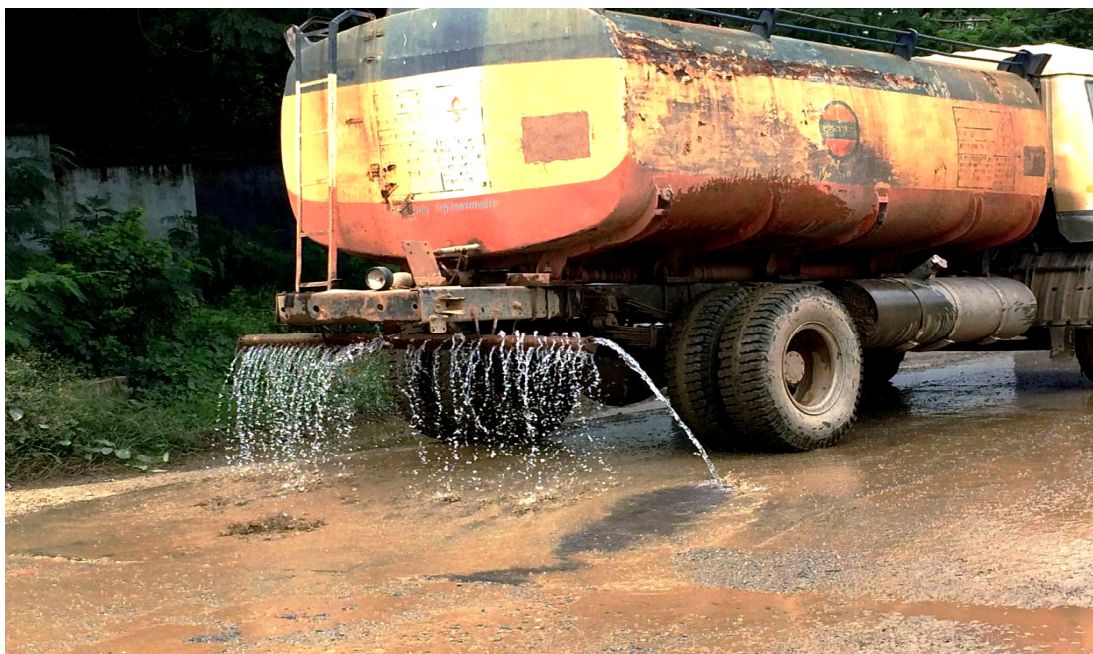
Photograph showing water sprinkling in haul road
